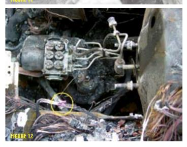
Based on the inspection so far, the investigator should have a working hypothesis about the origin of the fire at the Speed Control Deactivation Switch and be prepared to locate and document the switch remains.
