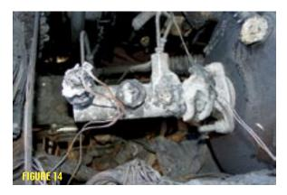
Often the electrical (base) portion of the switch will be detached from the hexport (body). The electrical portion may still be attached by the wiring or may have fallen to the inside of the driver's side front tire. A hexport with a detached electrical section may look like the one shown in Figure 15 (the electrical portion is hanging over the master cylinder and still attached by one wire).
